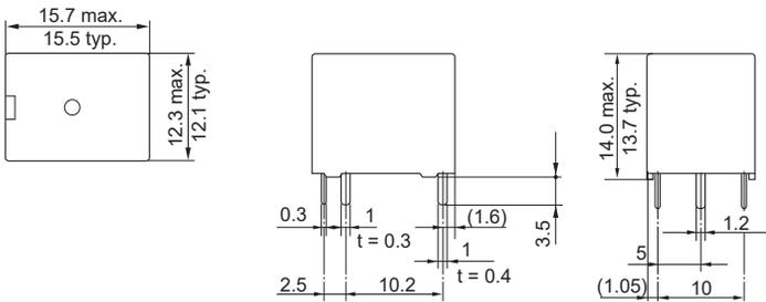
\* Dimensions of the terminals do not include thickness of pre-solder.
