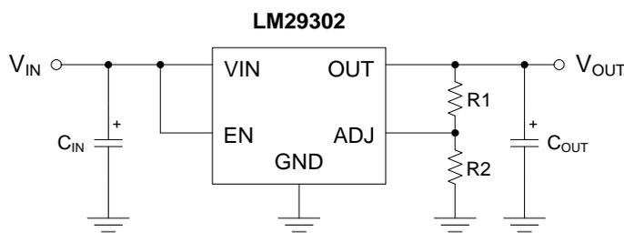
$$V_{OUT} = V_{REF} \times [1 + (R1/R2)] *$$
