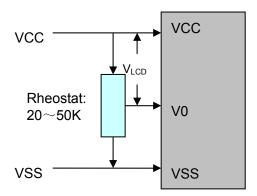
We recommend allowing field adjustment of V0 for all designs. The optimal value for V0 will change with temperature, variations in VDD, and viewing angle. V0 will also vary module-to-module and batch-to-batch due to normal manufacturing variations.
