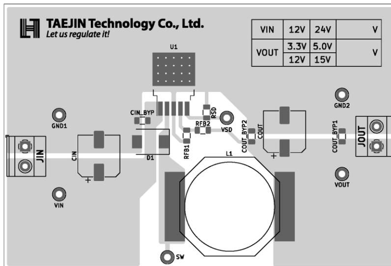
Figure 28. PCB Layout Example
