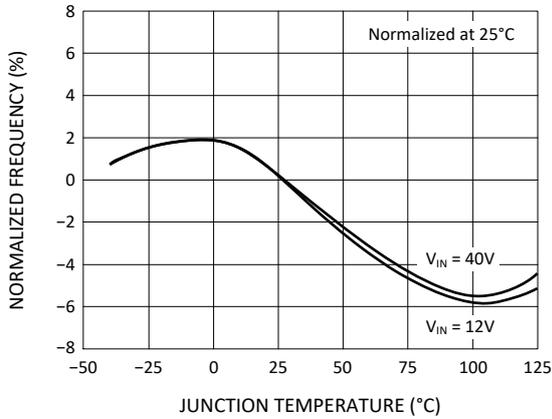
Figure 7. Oscillator Frequency
