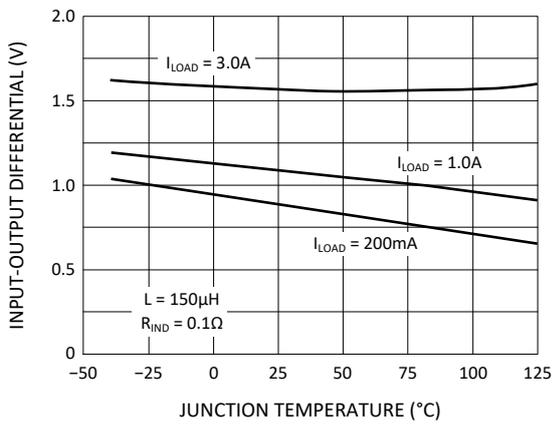
Figure 3. Dropout Voltage
