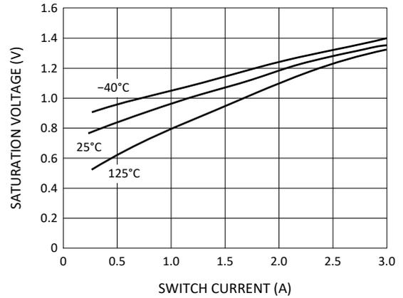
Figure 8. Switch Saturation Voltage
