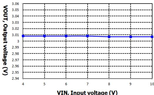
VIN=4.0V to 10V, VOUT=3.0V @ IOUT=10mA
