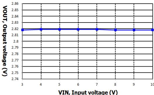
VIN=3V to 10V, VOUT=2.8V @ IOUT=10mA
