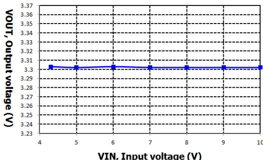
VIN=4.3V to 10V, VOUT=3.3V @ IOUT=10mA
