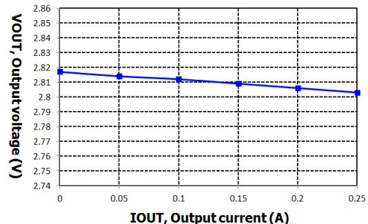
VIN=3.8V, VOUT=2.8V @ IOUT=250mA per 50mA step
