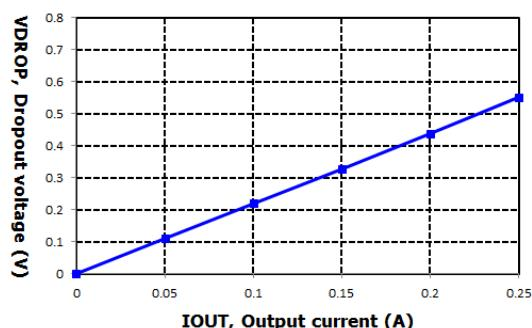
VIN=3.8V, VOUT=2.8V @ IOUT=250mA per 50mA step
