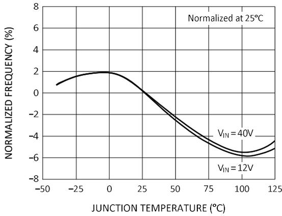
Figure 7. Oscillator Frequency
