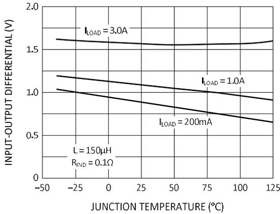
Figure 3. Dropout Voltage
