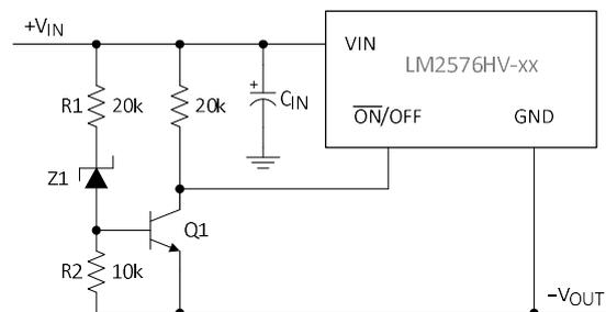
Figure 16. Undervoltage Lockout for Buck-Boost Circuit
