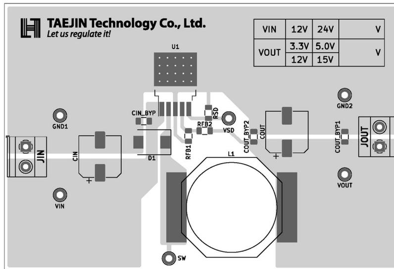
Figure 28. PCB Layout Example
