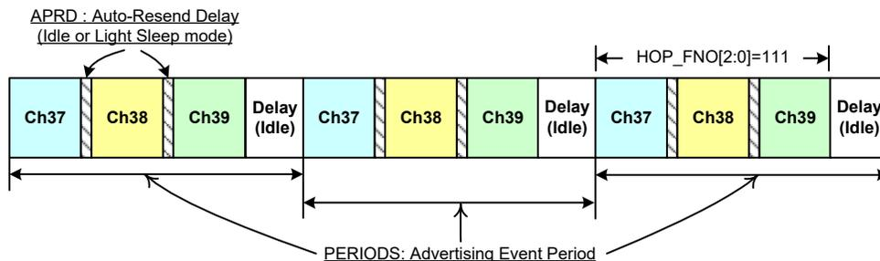
**PKT\_APRD[4:0]:** Packet format auto-resend delay, 250µs (Min.) ~ 8ms (Max.)
