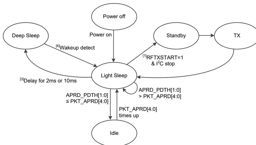
Note: 1. Once the RFTXSTART control bit is enabled, the I<sup>2</sup>C will stop and the RF chip will start transmitting data.
