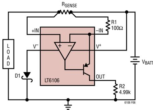
Figure 6. Schottky Diode Prevents Damage During Supply Reversal
