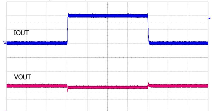
IOUT : 1.0A/div, VOUT : 100mV/div, Time : 500μs/div
