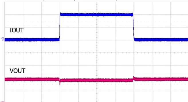
IOUT : 1.0A/div, VOUT : 100mV/div, Time : 500μs/div
