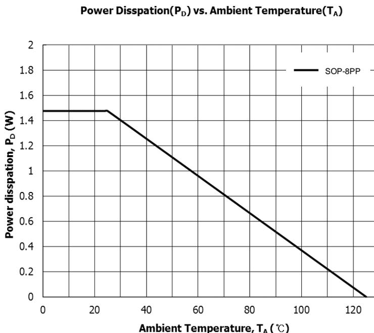
The graph above is valid for the thermal impedance specified in the Absolute Maximum Ratings section on page 1.
