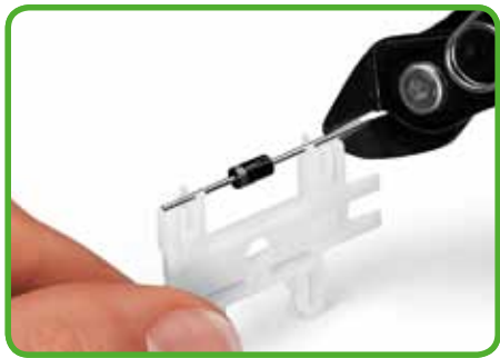
Measure component length with 2002-116 tool
