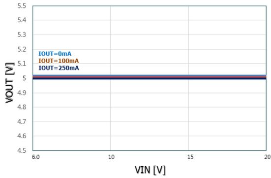
VIN=6.0V to 20V, VOUT=5.0V @ IOUT=0A/100mA/250mA
