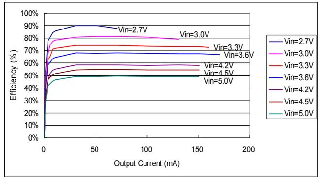
Fig. 14 Efficiency vs. Output Current
