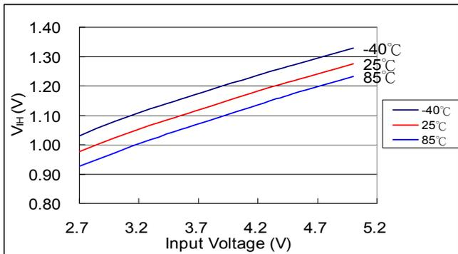
Fig. 15  $V_{IH}$  vs. Input Voltage
