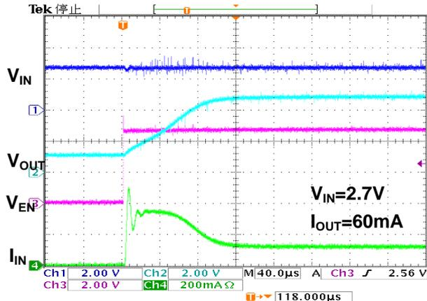
Fig. 18 Inrush Current ( $V_{IN}=2.7V$ ,  $I_{OUT}=60mA$ )
