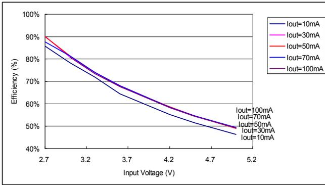
Fig. 13 Efficiency vs. Input Voltage
