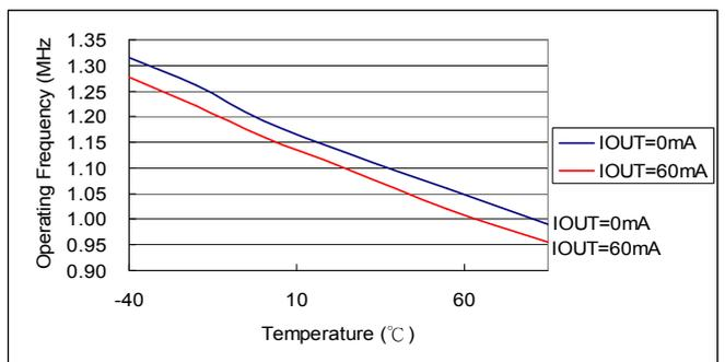
Fig. 12 Operating Frequency vs. Temperature ( $V_{IN}=3.7V$ )
