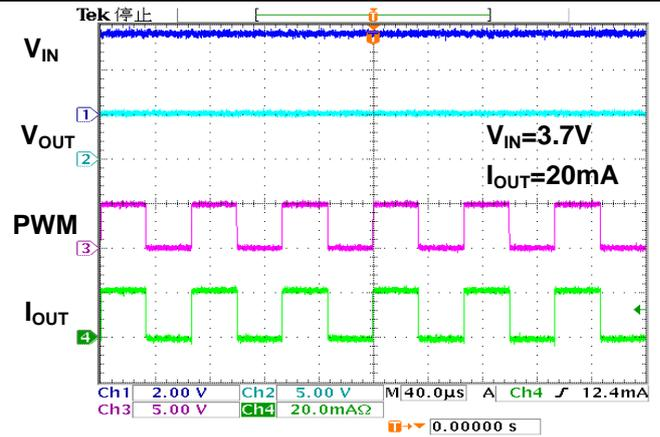
Fig. 25 Dimming Operation (Refer to Fig. 26)
