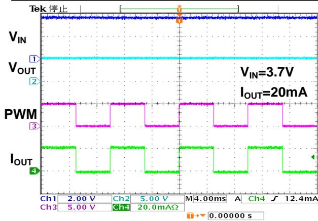
Fig. 24 Dimming Operation (Refer to Fig. 26)
