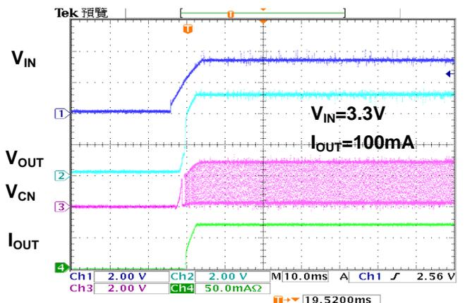
Fig. 23 Start-Up Waveform ( $V_{IN}=3.3V$ ,  $I_{OUT}=100mA$ )
