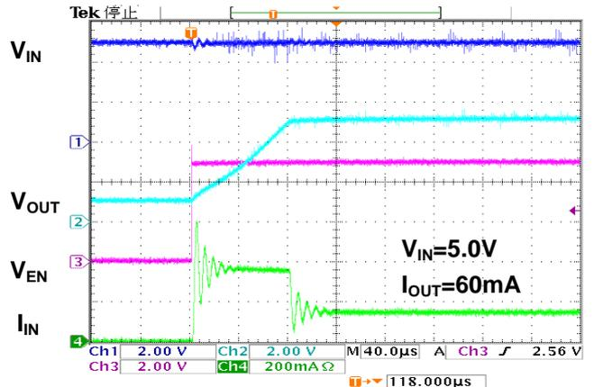
Fig. 19 Inrush Current ( $V_{IN}=5.0V$ ,  $I_{OUT}=60mA$ )
