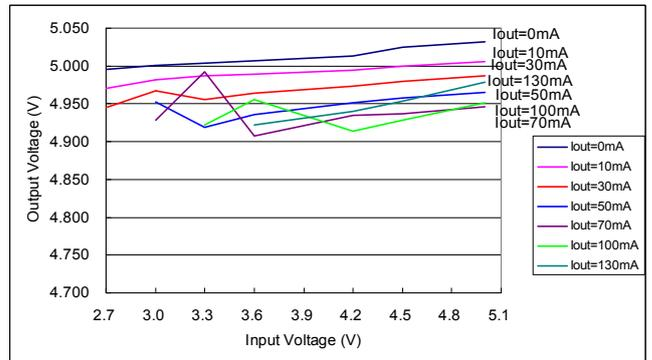
Fig. 8 Output Voltage vs. Input Voltage ( $C_{IN}=C_{OUT}=1\mu F$ ,  $C_{FLY}=0.1\mu F$ )
