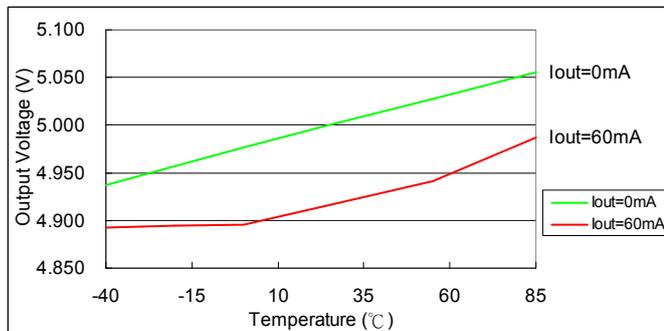
Fig. 11 Output Voltage vs. Temperature ( $V_{IN}=3.3V$ )
