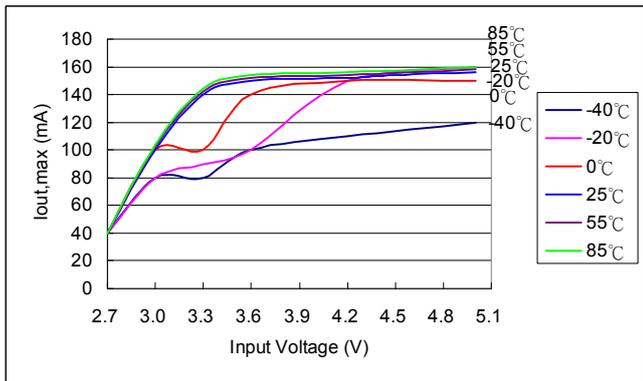
Fig. 17 Maximum Output Current vs. Input Voltage
