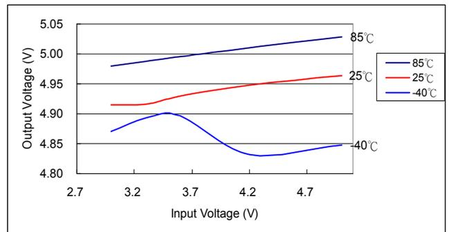
Fig. 10 Output Voltage vs. Input Voltage ( $I_{OUT}=60mA$ )
