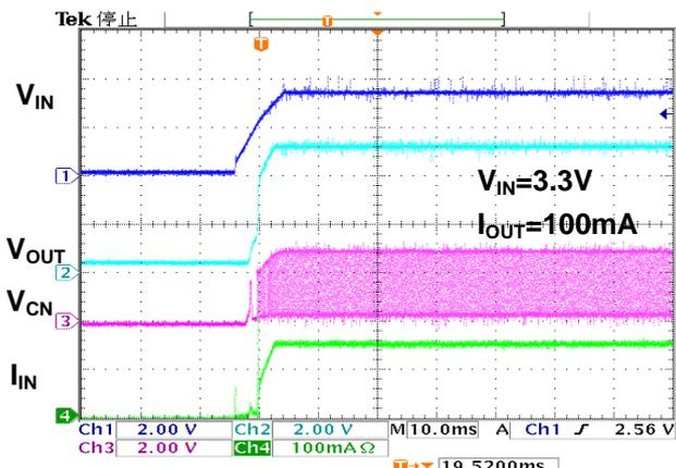
Fig. 22 Start-Up Waveform ( $V_{IN}=3.3V$ ,  $I_{OUT}=100mA$ )
