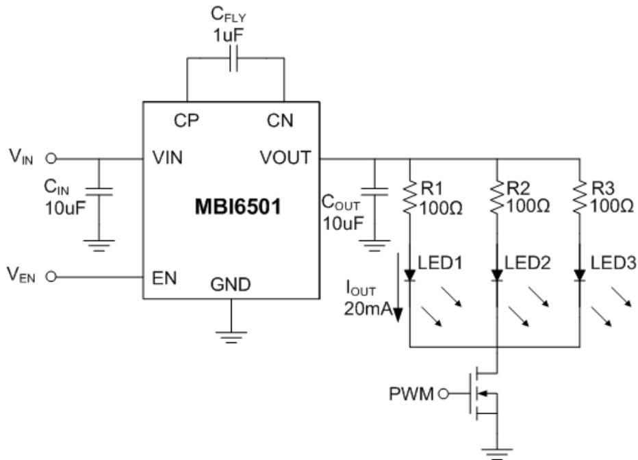
Fig. 26 Application circuit for backlight dimming
