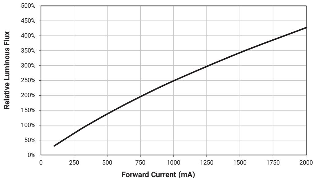
**RELATIVE RADIANT FLUX VS. CURRENT - COLOR ( $T_J = 25^\circ\text{C}$ )**
