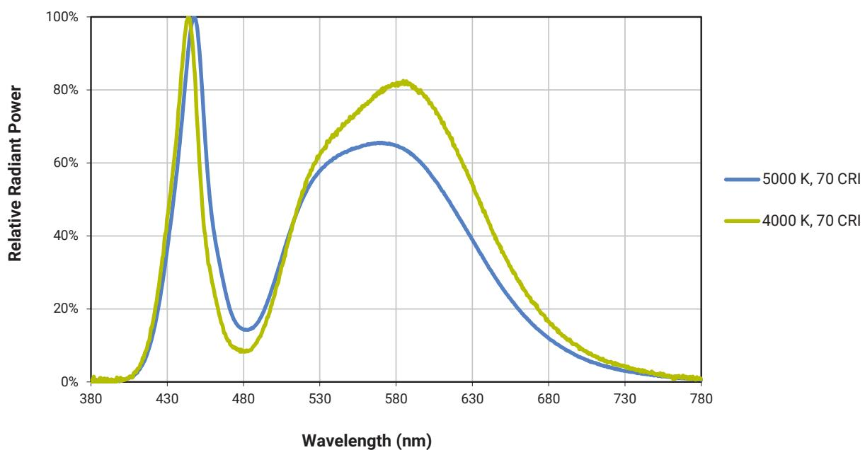
**RELATIVE SPECTRAL POWER DISTRIBUTION - COLOR**
