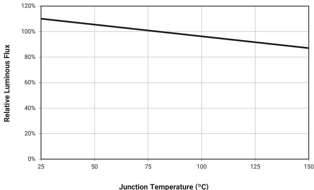
**RELATIVE FLUX VS. JUNCTION TEMPERATURE - COLOR -  $I_F = 350 \text{ mA}$**
